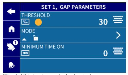
[Threshold] is the trigger point for signal points.
