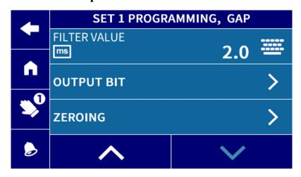
Click on 【OUTPUT BIT】 to set the idle output signal points
