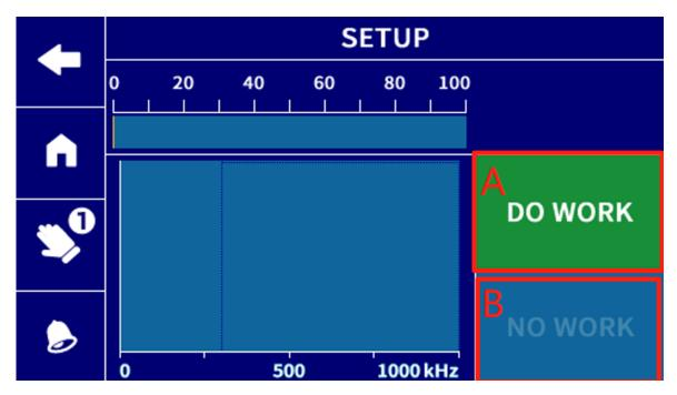
Area A corresponds to the contact between the grinding wheel and the workpiece, while Area B corresponds to the non-contact between the grinding wheel and the workpiece.
