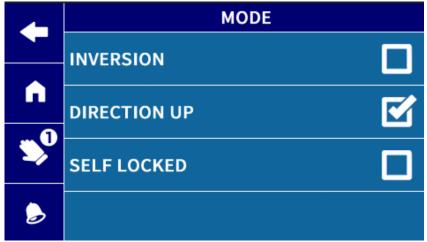
[INVERSION] Checking this option will cause the function to invert the state of the output signal based on the control logic conditions.
