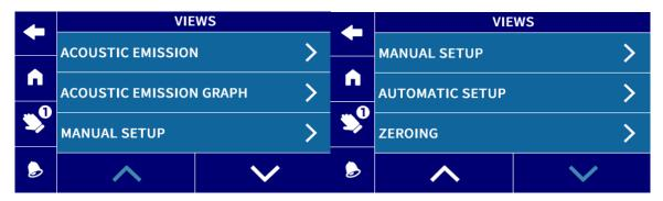
① 【ACOUSTIC EMISSION】 is the measurement monitoring interface, which allows viewing of measurement values and signal point status.
